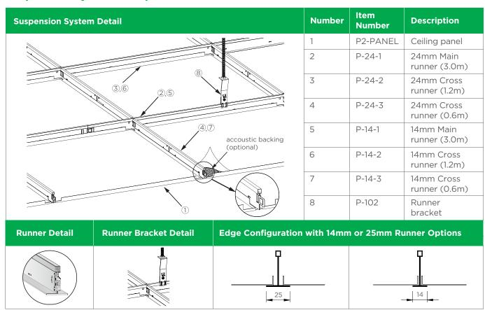
The suspension system consists of the T-shaped Main runners and Cross runners connected to the Runner bracket (8).
